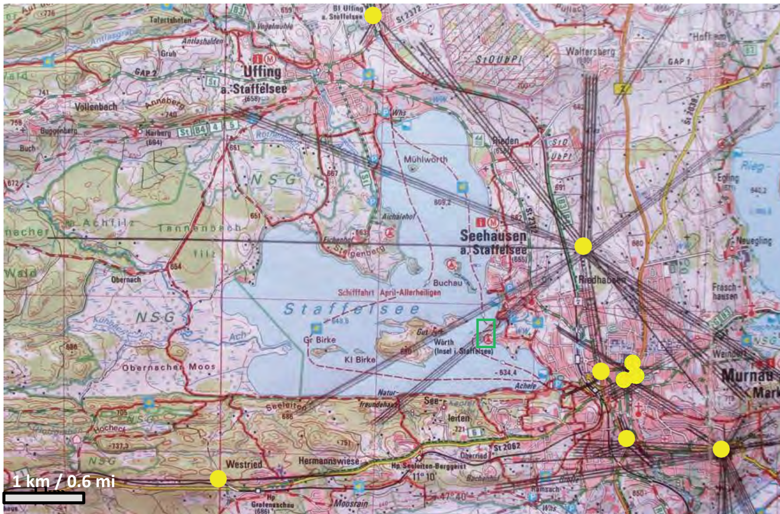
Section UK 50-49, Pfaffenwinkel, Bavarian State Agency for Digitization, High-Speed Internet and Surveying Added: locations of mobile phone base stations with the main beam directions of the sector antennas, camping site (green).
